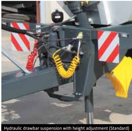
Hydraulic drawbar suspension with height adjustment (Standard)
