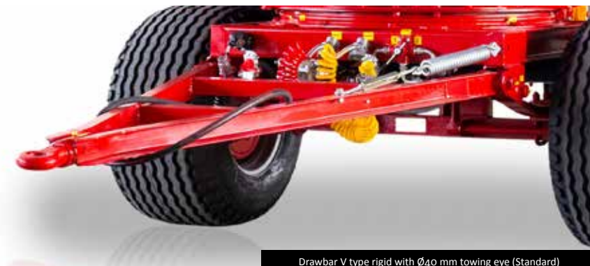
Drawbar V type rigid with Ø40 mm towing eye (Standard)
