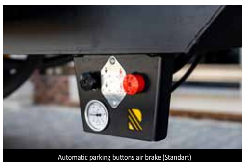
Automatic parking buttons air brake (Standart)
