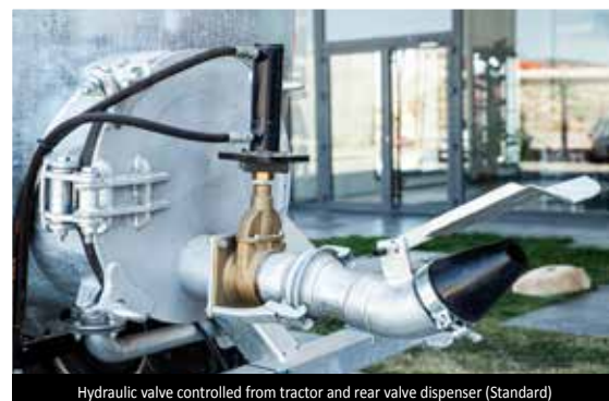
Hydraulic valve controlled from tractor and rear valve dispenser (Standard)
