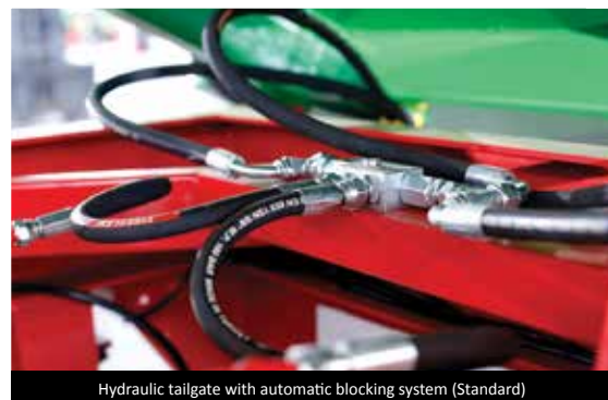
Hydraulic tailgate with automatic blocking system (Standard)
