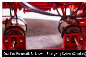
Dual Line Pneumatic Brakes with Emergency System (Standard)
