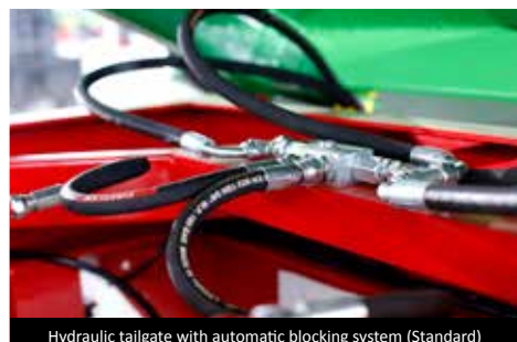
Hydraulic tailgate with automatic blocking system (Standard)
