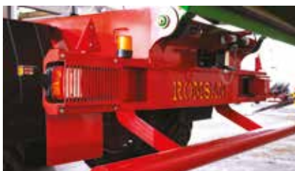
Tail lights with protective grating (Standard)
