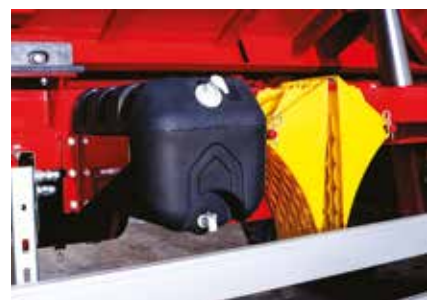
Water Tank (Optional) - Wheel Chocks (Standard)
