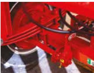
Parabolic Spring (Standart)
