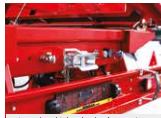
Manual rear hitch and outlets for secondary trailer (Standart)
