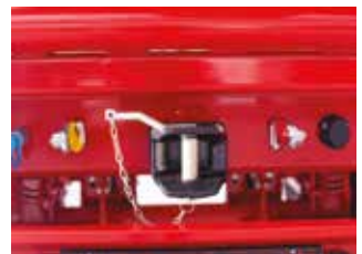
Rear Manual Hitch and outlets for secondary trailer (Optional)
