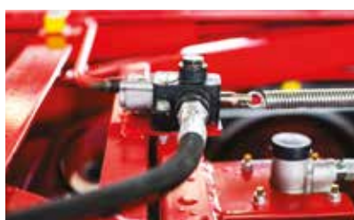
Hydraulic tipping system with cut-off valve (Standard)
