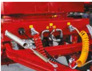
Height adjustment spring for drawbar (Standart)
