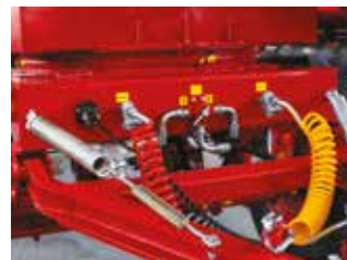
Height adjustment spring for drawbar (Standart)
