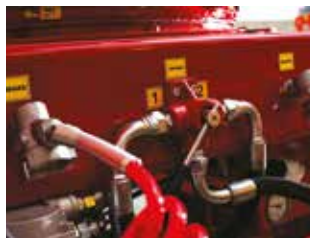
Hydraulic controllers for secondary trailer (Standart)
