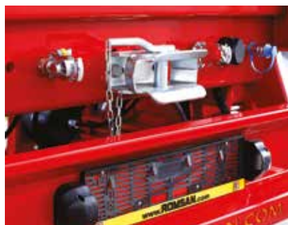
Manual rear hitch and outlets for secondary trailer (Optional)
