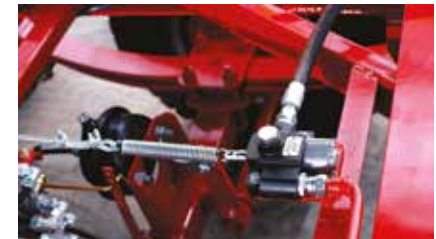
Hydraulic tipping system with cut-off valve (Standard)
