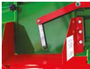
Rear grain chute (Standart)
