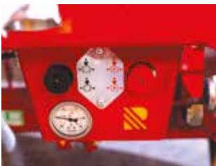
Automatic parking buttons air brake (Standart)
