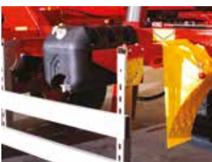
Water Tank and Wheel Chocks (Standart)
