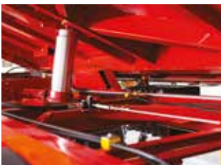
Hydraulic tipping system with cut-off valve (Standard)
