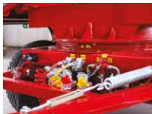
Height adjustment spring for drawbar (Standard)
