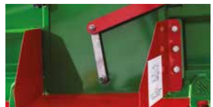
Rear grain chute (Standard)
