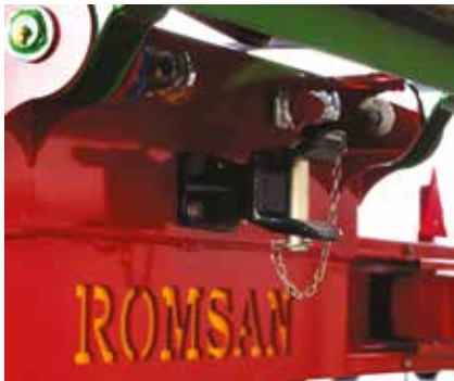
Rear Manual Hitch and outlets for secondary trailer (Optional)
