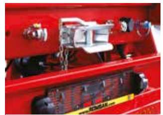
Manual rear hitch and outlets for secondary trailer (Optional)
