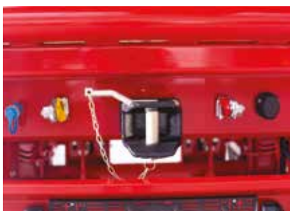
Rear Manual Hitch and outlets for secondary trailer (Optional)
