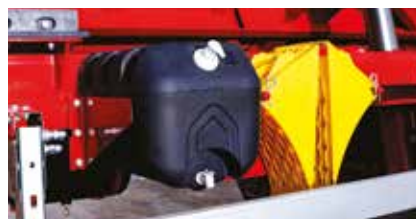
Water Tank (Optional) - Wheel Chocks (Standard)
