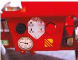
Automatic parking buttons air brake (Standart)
