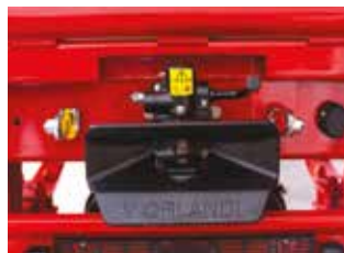
Rear automatic hitch and outlets for secondary trailer (Optional)
