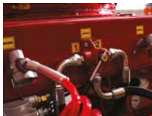
Hydraulic controllers for secondary trailer (Standart)
