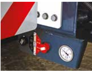
Automatic parking buttons air brake (Standart)
