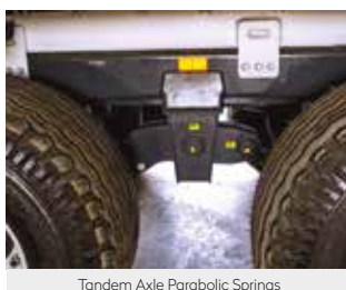
Tandem Axle Parabolic Springs
