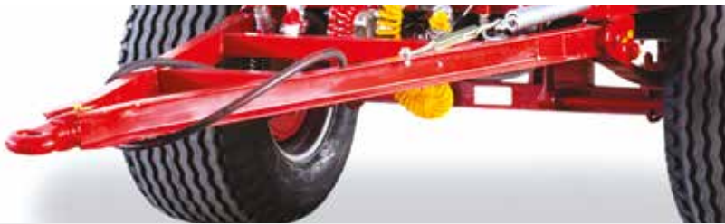
Drawbar V type rigid with Ø40 mm towing eye (Standard)
