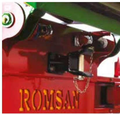
Rear Manuel Hitch and outlets for secondary trailer (Optional)
