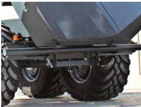
Tail lights with protection bar during operation (Standard)
