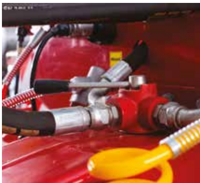
Hydraulic controllers for secondary trailer (Optional)
