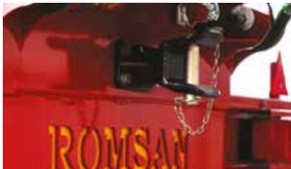
Rear Manual Hitch and outlets for secondary trailer (Optional)
