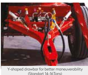
Y-shaped drawbar for better maneuverability (Standart 14-16Tons)
