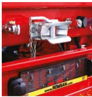
Manuel rear hitch and outlets for secondary trailer (Optional)
