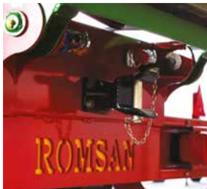
Rear Manuel Hitch and outlets for secondary trailer (Optional)
