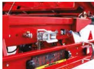
Manual rear hitch and outlets for secondary trailer (Standard)
