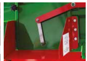
Rear grain chute (Standard)
