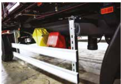
Side underrun protection and Wheel Chocks racks (Standard) Fire Box (Optional)
