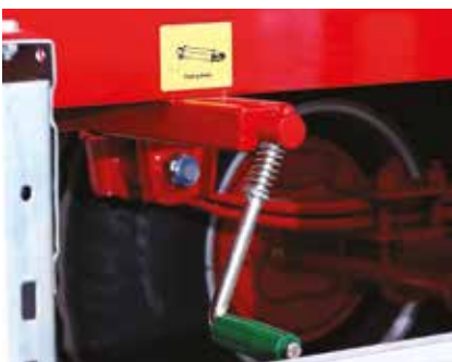
Parking brake (Handbrake) (Standard)
