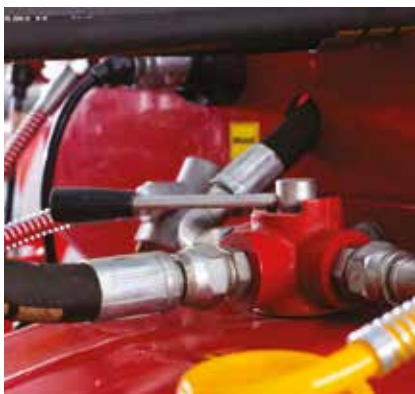
Hydraulic controllers for secondary trailer (Optional)
