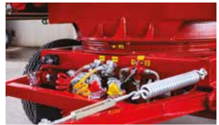
Height adjustment spring for drawbar (Standard)
