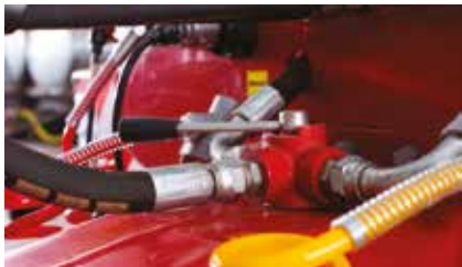
Hydraulic controllers for secondary trailer (Optional)
