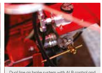
Dual line air brake system with ALB control and air parking brake with emergency (Standart)
