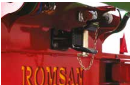
Rear Manuel Hitch and outlets for secondary trailer (Optional)
