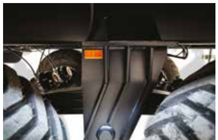
Reverse Parabolic Spring yering tandem bogie system (Standard)
