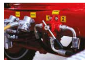
Hydraulic controllers for second trailer (Standard)
