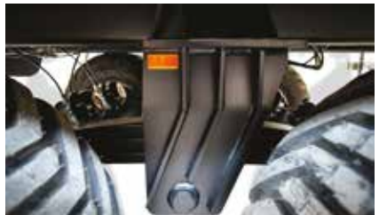
Reverse Parabolic Spring yerine tandem bogie system (Standard)
