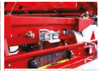
Manuel rear hitch and outlets for secondary trailer (Standart)
