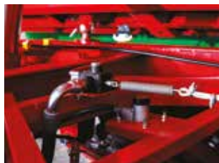
Hydraulic tipping system with cut-off valve (Standard)
