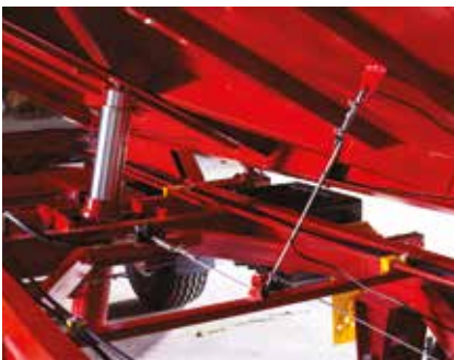
Hydraulic tipping system with cut-off valve (Standard)
