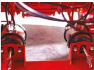
Dual Line Pneumatic Brakes with Emergency System (Standard)
