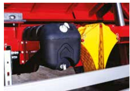
Water Tank (Optional) Wheel Chocks (Standard)
