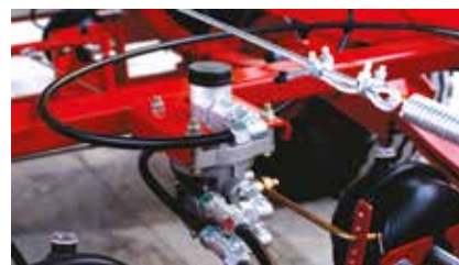
Dual line air brake system with ALB control and air parking brake with emergency (Standard)
