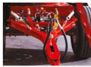
Y-shaped drawbar for better maneuverability (Standart 14-16Tons)
