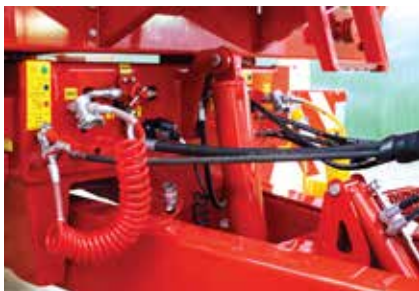
Hydraulic Jack For Drawbar (Standard)
