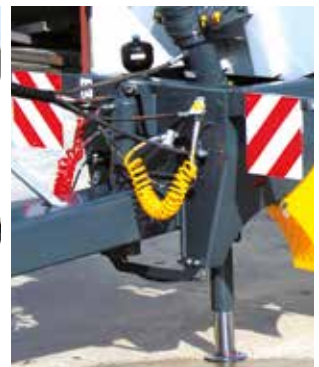
Hydraulic drawbar suspension with height adjustment (Standard)
