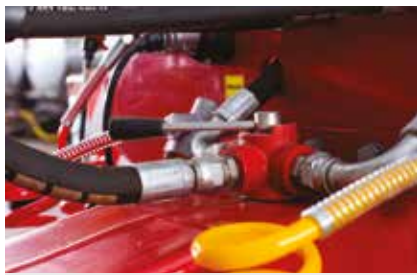
Hydraulic controllers for secondary trailer (Optional)
