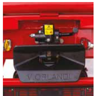
Rear automatic hitch and outlets for secondary trailer (Optional)
